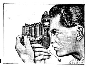
maintained. The various markings are set opposite the indication by revolving the milled ring 8. All shutters are released by pressing down the trigger 16 (fig. 1), which operates the release lever.
