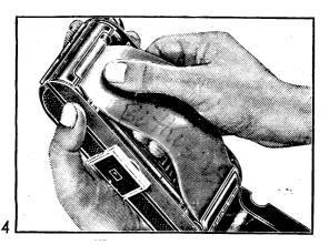
First insert the mask at the bottom, then bend gently and let it spring in at the top. It must then lie absolutely flat. When closing the camera back, the upper film window, which is closed with full size  $6 \times 9 \, \text{cm}$ , opens
